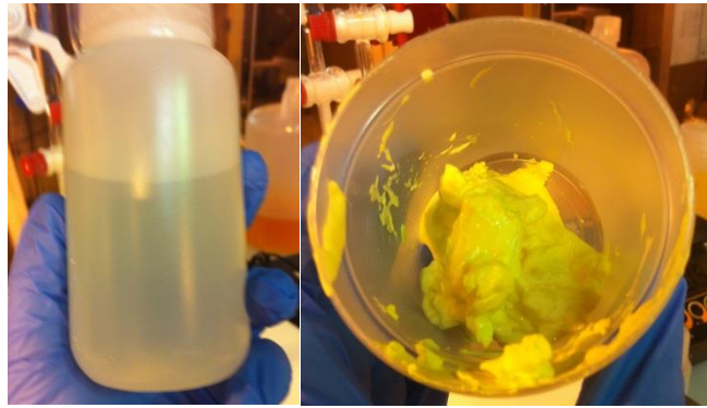
Figure 4.24 – First Test Series, Auxiliary Testing, \text{UO}_4 (yellow solids) and filtrate (clear liquid)
