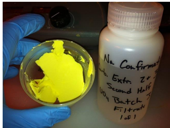
Figure 4.48 – Fifth Test Series, Batch 3, UO 4 filter cake (left) and filtrate (right).
