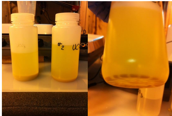
Figure 4.16 – Final \text{UCO}_3 Products. Clear, yellow uranyl carbonate solution, with thin layers of brown sediment (most likely iron carryover).
