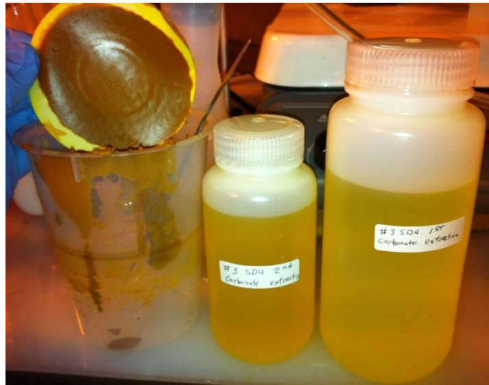
Figure 4.39 – Fifth Test Series SDU Carbonate Extraction 2. Residual solids on the left and carbonate extractions #2 and #1 on the right.
