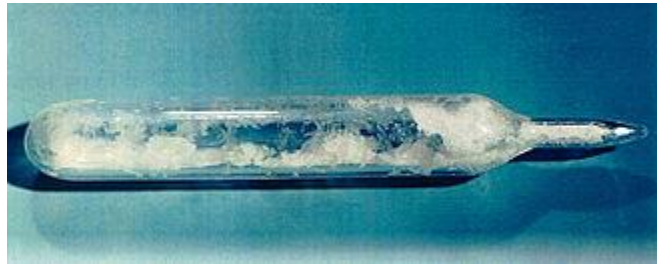
Figure 1.2 – UF 6 crystals in a small glass ampoule (4)
