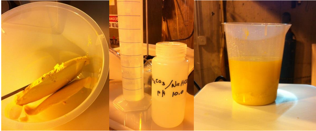
Figure 4.14 – SDU Filter Cake in Beaker, Sodium Carbonate/Bicarbonate mixture (pH=10), Slurry of SDU and 300 mL of 10% \text{Na}_2\text{CO}_3 solution
